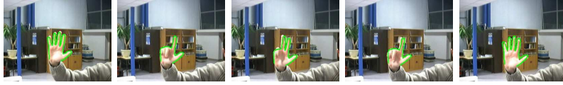
Fig. 6. “Interaction through commanding gestures”: hand configurations tracking on a sequence involving cluttered background when fusing color and shape cues in the particles likelihood.
