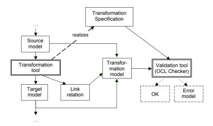
Fig. 5. High-level view of model transformation and verification
