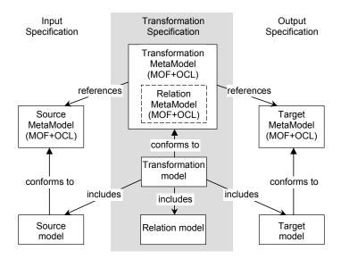
Fig. 4. High level view of the model transformation specification
