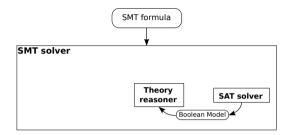
Input:  $a \leq b \wedge b \leq a + x \wedge x = 0 \wedge [f(a) \neq f(b) \vee (q(a) \wedge \neg q(b+x))]$ To SAT solver:  $p_{a \leq b} \wedge p_{b \leq a+x} \wedge p_{x=0} \wedge [\neg p_{f(a)=f(b)} \vee (p_{q(a)} \wedge \neg p_{q(b+x)})]$ Boolean model:  $p_{a \leq b}, p_{b \leq a+x}, p_{x=0}, \neg p_{f(a)=f(b)}$ Theory reasoner:  $a \leq b, b \leq a + x, x = 0, f(a) \neq f(b)$  unsatisfiable
