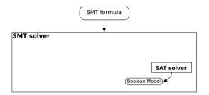
Input:  $a \leq b \wedge b \leq a + x \wedge x = 0 \wedge [f(a) \neq f(b) \vee (q(a) \wedge \neg q(b+x))]$ To SAT solver:  $p_{a \leq b} \wedge p_{b \leq a+x} \wedge p_{x=0} \wedge [\neg p_{f(a)=f(b)} \vee (p_{q(a)} \wedge \neg p_{q(b+x)})]$ Boolean model:  $p_{a \leq b}, p_{b \leq a+x}, p_{x=0}, \neg p_{f(a)=f(b)}$
