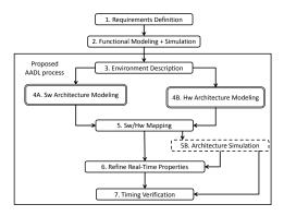
Fig. 1. Proposed Design Flow
