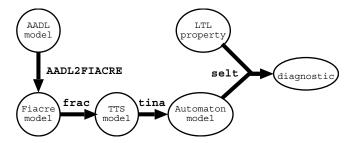
Fig. 5. The verification process.
